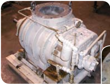
The blower arrives at the shop with product contamination.
