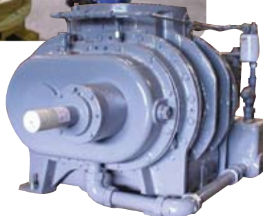
After a thorough inspection, the technician will clean, repair, test, and then paint the blower before returning it to the customer with a full one year warranty.
