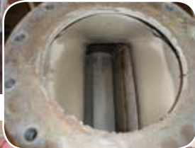
The blower arrives at the shop with product contamination.
