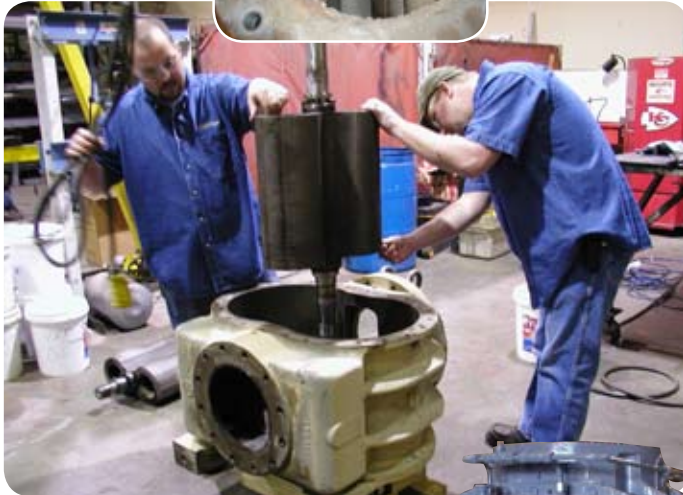
After a thorough inspection, the technician will clean, repair, test, and then paint the blower before returning it to the customer with a full one year warranty.
